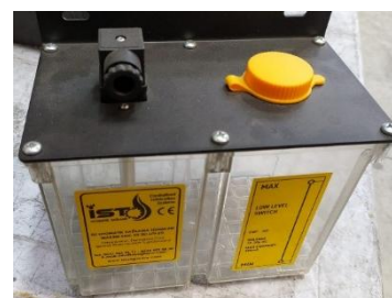
Figure 4 Oil tank with level sensor
